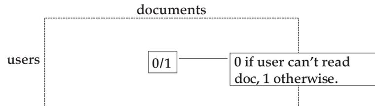
► **Figure 4.8** A user-document matrix for access control lists. Element  $(i, j)$  is 1 if user  $i$  has access to document  $j$  and 0 otherwise. During query processing, a user's access postings list is intersected with the results list returned by the text part of the index.
