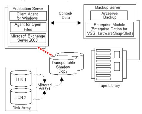
**Note:** The dashed line represents the logical connection between a Microsoft Exchange 2003 Server and the cloned data on the transportable shadow copy volume.
