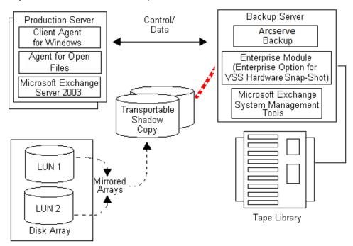
**Note:** The dashed line now represents the logical attachment between the Arcserve Backup server and the cloned data on the transportable shadow copy volume.
