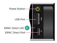
The iDRAC Direct LED indicator lights up to indicate that the port is connected and is being used as part of the iDRAC subsystem.
