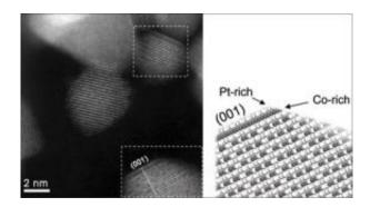
Left image highlights two platinum-cobalt catalyst nanoparticles (inside the dashed boxes) with a 'sandwich' structure of platinum and cobalt atoms near the surface. At right is a cross-sectional model corresponding to the lower particle, showing platinum atoms enriched in the outermost layer, cobalt enriched in the second, and additional layers containing a mixture of the two. (Image at left taken at Oak Ridge National Laboratory.) Image courtesy / Electrochemical Energy Laboratory at MIT
