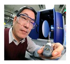
Materials engineer Duck Young Chung examines a sample of superconducting crystals before characterizing them in a X-ray diffractometer. The crystals signify the next generation of experiments utilizing neutron scattering to determine unconventional superconductivity.
