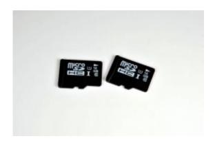
Samsung Electronics today announced that it is now mass producing Ultra High Speed–1 (UHS-1) interface microSD cards that support the highest performance levels required on advanced LTE (Long Term Evolution) smartphones and tablets.
