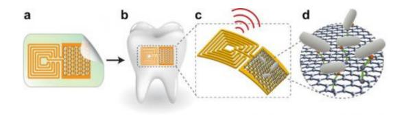
The sensor (A), attached to a tooth (B) and activated by radio signals (C), binds with certain bacteria (D). Credit: Manu Mannoor/Nature Communications
