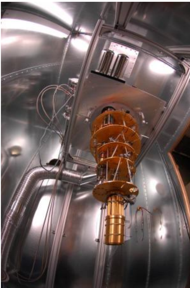
The D-Wave Systems Fridge with Cryogenic Packaging
