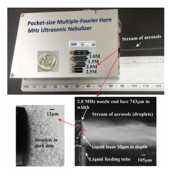
This is a pocket-size ultrasonic nebulizer with insets: (Top) Nebulizer and MEMS-fabricated MHz nozzles laid on its cover. (Bottom) Aerosols ejected from the medicinal liquid layer resting on the end face of the nozzle tip: (L) Individual aerosols imaged using a high-speed camera (104 frame/sec) with short
