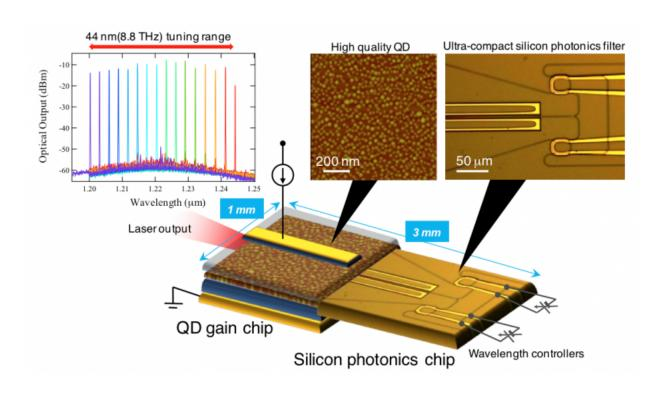
The novel heterogeneous wavelength tunable laser diode consists of QD technology and silicon photonics. Credit: Tomohiro Kita
