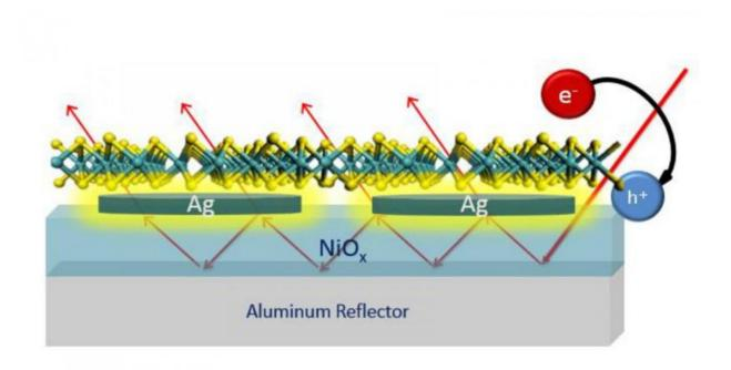
Using a layer of molybdenum disulfide that was less than one nanometer thick, researchers in Rice University's Thomann lab were able to design a system that absorbed more than 35 percent of incident light in the 400- to 700-nanometer wavelength range. Credit: Thomann Group/Rice University
