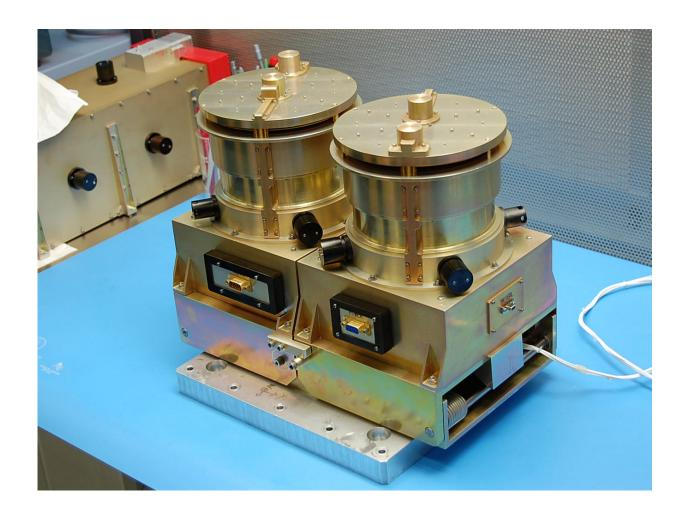
Goddard is providing MILENA, which is short for Miniaturized Imager for Low-Energy Neutral Atoms, as one of five payloads on the VISIONS-2 soundingrocket mission. It traces its heritage to an instrument that flew on the U.S. Air Force-sponsored FASTSAT mission in 2011. Credit: NASA
