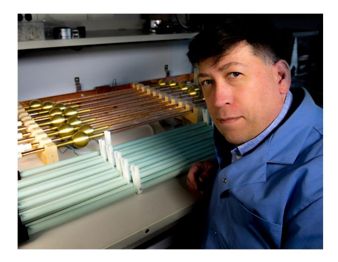
Principal Investigator Doug Rowland is pictured here with electric-field booms that flew on VISIONS-1. His follow-on sounding-rocket mission will fly similar booms to measure the electric fields that energize oxygen ions and accelerate them against Earth's gravity. Credit: : NASA/W. Hrybyk
