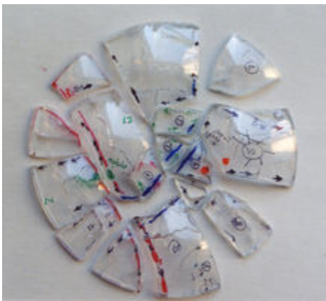
Fracture of a sapphire dome. Credit: NIST
