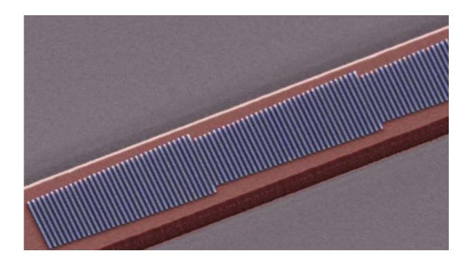
Image of a fabricated device showing four phased antenna arrays consisting of silicon nano-rods of different lengths patterned on the top surface of a LiNbO3 waveguide. Credit: Loncar Lab/Harvard SEAS
