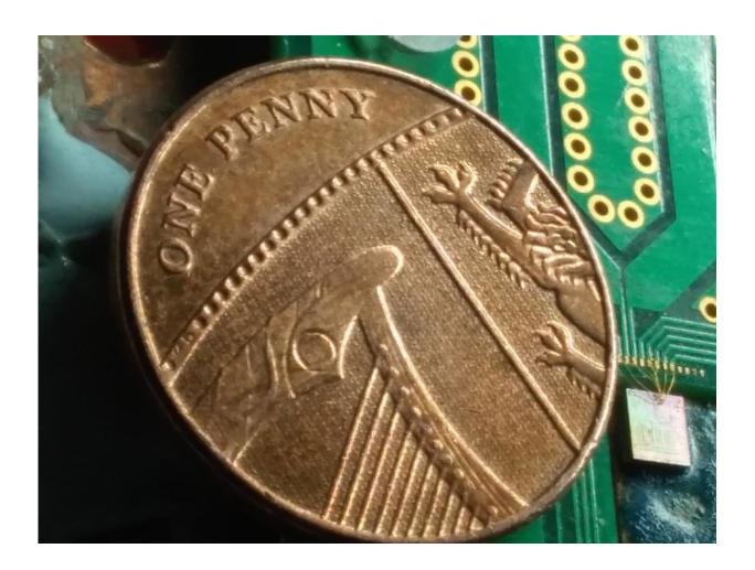
Researchers created a chip-based device measuring a millimeter square that can potentially generate quantum-based random numbers at gigabit per second speeds. The small square to the right of the penny contains all the optical components of the random number generator. Credit: Francesco Raffaelli,
