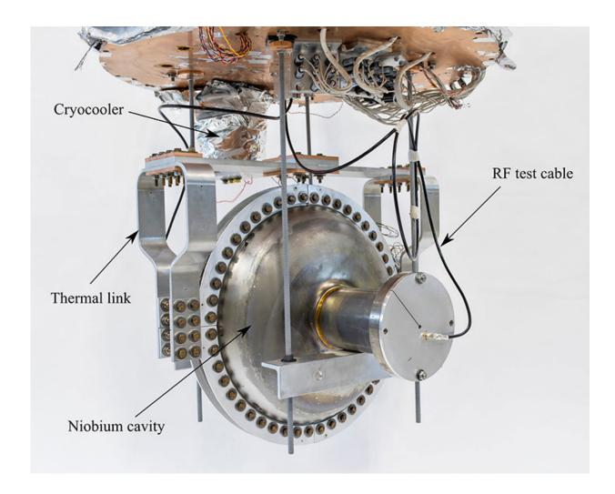
A superconducting radio-frequency (RF) accelerator cavity is mounted and connected to a cryocooler, cooling the cavity without the use of liquid helium. This new device could make it easier to produce high-average-power electron beams for industrial applications. Credit: US Department of Energy
