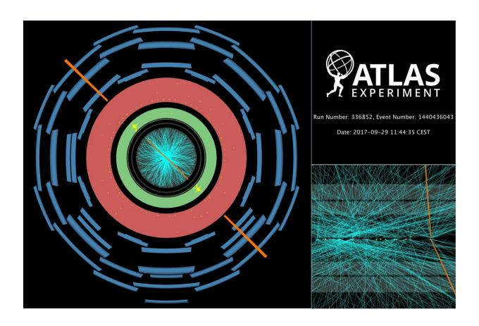
Display of a candidate event for new heavy particles decaying into two electrons in the ATLAS Experiment. Credit: ATLAS Collaboration/CERN
