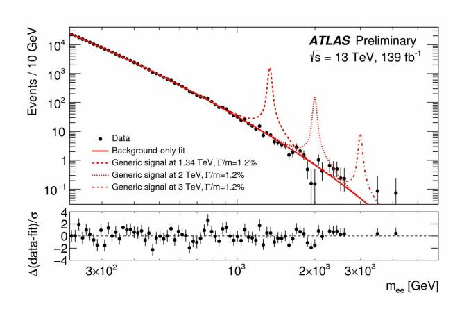
Measured dielectron mass distribution for the data (black points), together with the total background fit result is shown (red continuous line), with various possible Z' signal distributions overlaid (dashed red line). The sub-panel shows the significance of the deviation between the observed data and the background prediction in each bin of the distribution. Credit: ATLAS Collaboration/CERN
