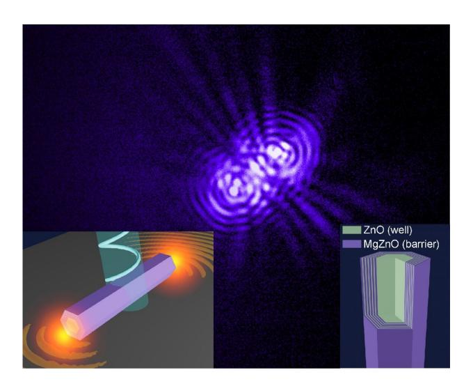
Coherent light emission of one-dimensional polaritons in the quantum well nanocavity. Above the lasing threshold, the interference pattern, which is associated with Fabry-Pérot cavity modes along the long axis of the nanorod (left inset), is observed. The radial quantum wells integrated on the sidewall of the nanorod (right inset) provide the enhanced thermal stability and oscillator
