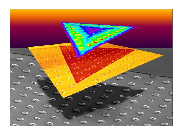
Strain-tolerant, triangular, monolayer crystals of WS2 were grown on SiO2 substrates patterned with donut-shaped pillars, as shown in scanning electron microscope (bottom) and atomic force microscope (middle) image elements. The curvature of the pillars induced strain in the overlying crystals that locally altered their optoelectronic properties, as shown in bright regions of photoluminescence (top). Credit: Christopher Rouleau/Oak Ridge National Laboratory, US Dept. of Energy
