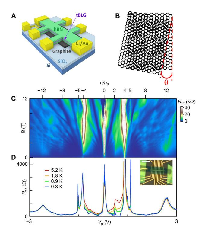
Device geometry and magneto-transport data. (A) Schematic diagram of device geometry. (B) Schematic diagram of moiré superlattice formed by the twisted graphene layers. (C) Rxx versus magnetic field B and gate voltage Vg showing a Landau fan pattern. The top axis labels nm, the number of charges per
