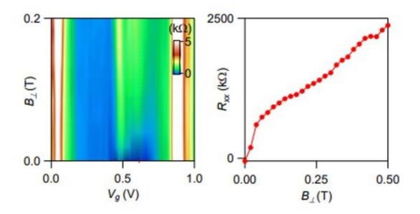
Superconductivity response to magnetic field. Rxx (Vg, B?) illustrating the disappearance of superconductivity with perpendicular magnetic field. Credit: Science Advances, doi: 10.1126/sciadv.aaw9770
