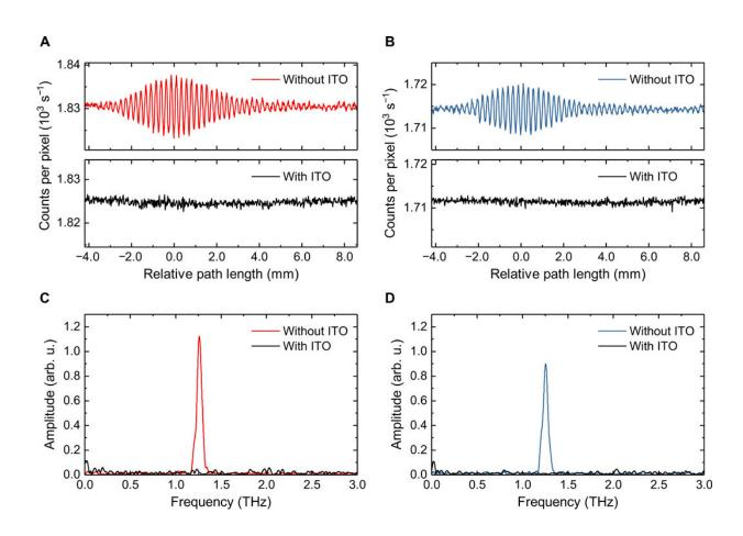
Terahertz quantum interference. In the collinear forward spot of the signal, interference is observed in the (A) Stokes and (B) anti-Stokes regions. (C and D) Corresponding FFTs peaks at about 1.26 THz. By placing an additional ITO glass in the idler path, no interference can be observed, and the peaks in the FFTs disappear. Credit: Science Advances, doi: 10.1126/sciadv.aaz8065
