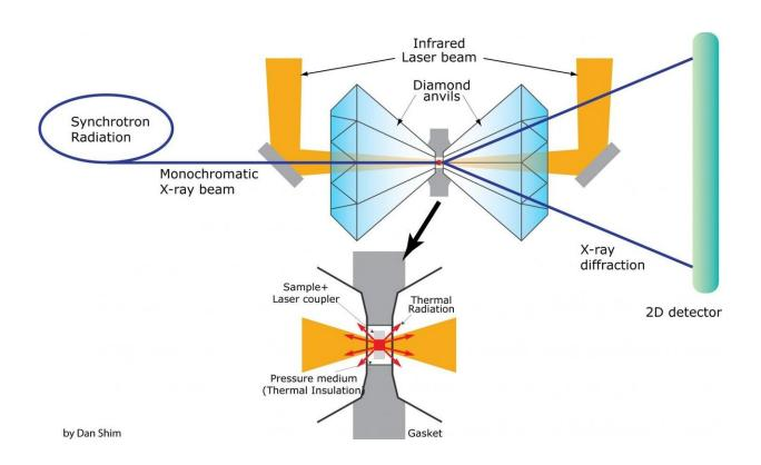
To measure crystal structures at the atomic scale at high pressure and temperature, a diamond-anvil cell with a sample is aligned with an X-ray beam (blue line) and laser beams (orange areas). The laser beams heat the sample to thousands of kelvins in temperature. The small red/gray rectangle sandwiched between diamond anvils is the sample. Credit: Dan Shim/ASU
