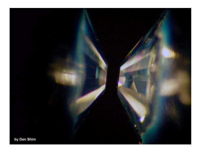
In a diamond-anvil cell, two gem quality single crystal diamonds are shaped into anvils (flat top in the photo) and then faced with each other. Samples are loaded between the culets (flat surfaces), then the sample is compressed between the anvils. Credit: Dan Shim/ASU
