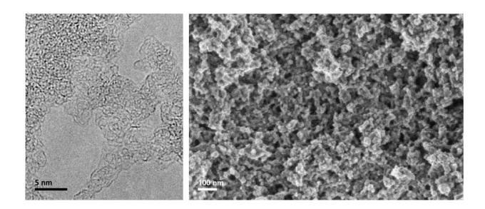
Electron microscopy images of the artificial cosmic dust grains, at different resolutions (transmission electron microscopy on the left, scanning electron microscopy on the right). Both show the complex, intricate surface structures of the grains, resulting in large surfaces. Credit: C. Jäger / MPIA und FSU Jena
