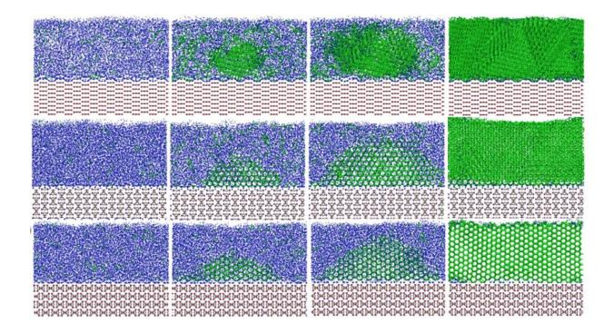
Simulations showing water molecules (blue) ordering into an ice crystal lattice (green) on different faces of a phloroglucinol crystal. Credit: Valeria Molinero/University of Utah
