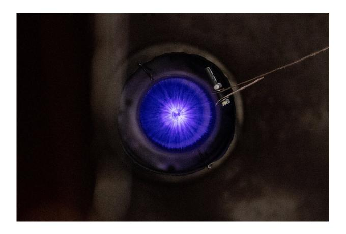
Electron beam irradiation with a dose  $\geq 5$  kGy is sufficient for full disinfection of the egg surface. Credit: UrFU / Ilya Safarov
