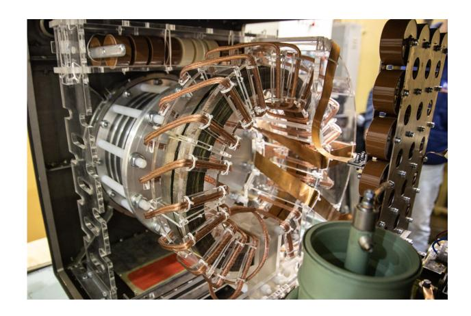
Irradiation experiments were carried out by the means of the URT-0.5 accelerator. Credit: UrFU / Ilya Safarov
