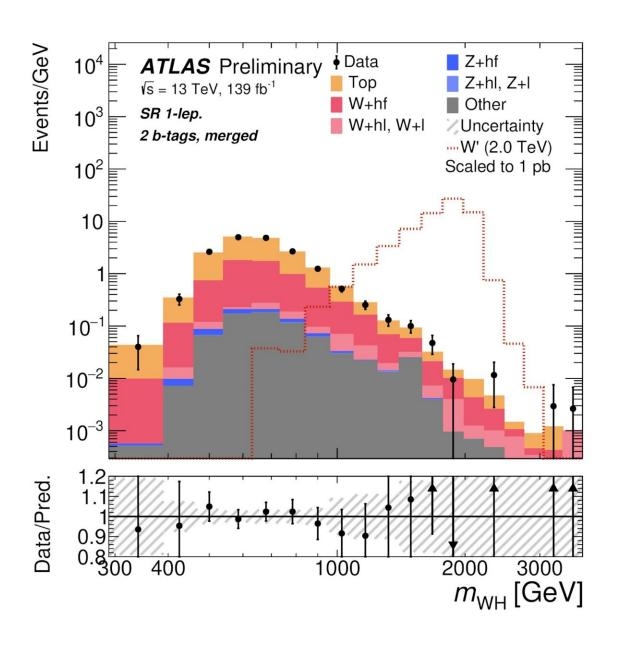
Figure 1: Post-fit distributions of the combined mass of the W boson and Higgs boson candidates in one signal region of interest for W'. (Here the 2 b-tag, merged region.) The solid colored region indicates the Standard Model background, the black points with error bars indicate the experimental data, and the dashed line indicates hypothetical events for a 2 TeV W' boson. The bottom plot shows the ratio of data to the total Standard Model background. Credit: ATLAS Collaboration/CERN
