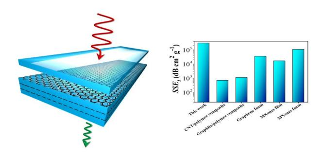
Sketch of the CVD graphene/polymer nanolaminates for EMI shielding. Credit: Foundation for Research and Technology - Hellas
