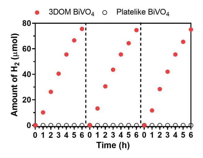
Plate-like bismuth vanadate produces negligible hydrogen, but 3DOM bismuth vanadate produces hydrogen under visible-light illumination. Credit: Hao Wu, Rowshanak Irani, Kunfeng Zhang, et al
