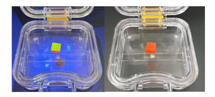
CH3NH3PbBr3 (MAPbBr3) monocrystal imaging under UV light and under visible ambient ligh. Credit: Arthur Ishteev
