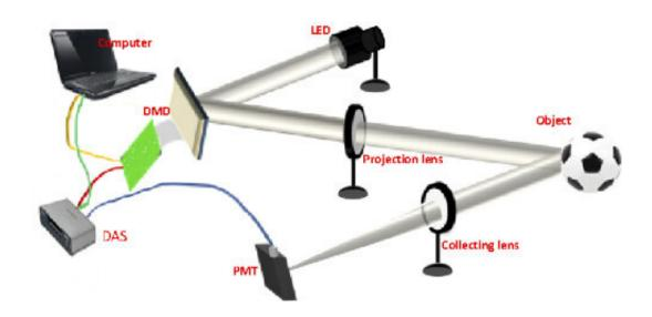
Experimental system. DMD is for digital micromirror device, LED is for light-emitting diode, PMT is for photomultiplier tube, and DAS is for data-acquisition system. Credit: Shi Dongfeng
