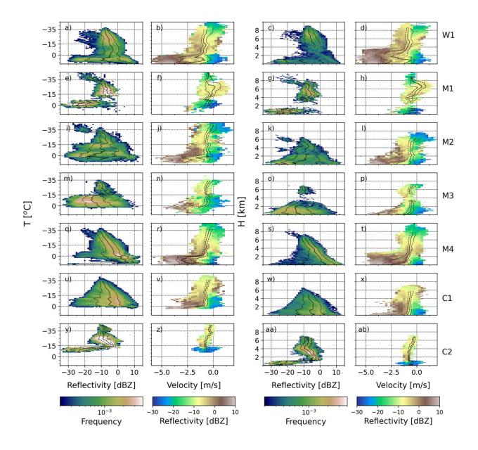
From left to right Bistatic Radar System for Atmospheric Studies cloud radar reflectivity Contour Frequency by Temperature Diagram and reflectivity median value as a function of temperature and Doppler velocity, followed by the same
