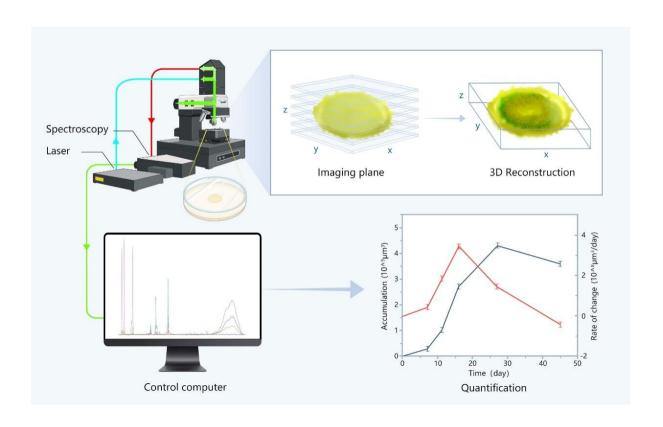
Schematic diagram of 3D quantitative imaging of colonies on solid medium. Credit: IOCAS
