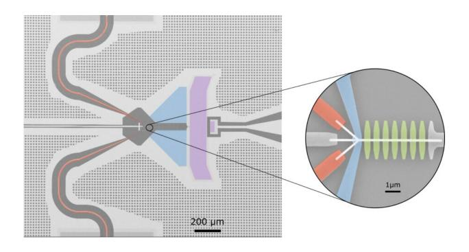
Image of the power sensor on a silicon chip. Credit: Jean-Philippe Girard/Aalto University
