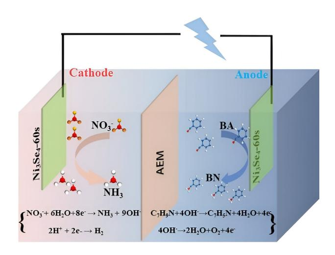
The Ni<sub>3</sub>Se<sub>4</sub> high-efficiency bifunctional electrocatalyst with Se vacancy was used for paired electrolysis of nitrate reduction and benzylamine oxidation in anion exchange membrane electrolyzer. Credit: Science China Press
