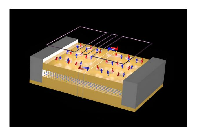
A schematic image showing a Josephson junction (central section) made from a single layer of tungsten telluride. The red spheres are electron with spin up, while the blue ones have spin down. Credit: RIKEN Advanced Device Laboratory
