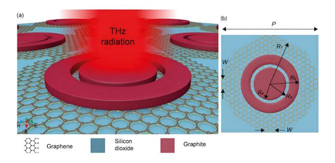
Thanks to its highly symmetrical structure, combined with optimized geometric parameters and material selection, the proposed tunable carbon-based terahertz absorber could lead to substantial advances and new applications in THz technology. Credit: Nie, He, and Cao, doi 10.1117/1.APN.3.1.016007.
