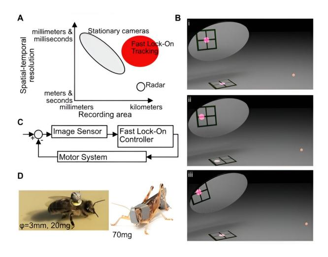
Fast lock-on tracking bypasses tradeoffs of other insect tracking techniques. (A) Conceptual view of tracking systems based on stationary cameras, radar, and Fast Lock-On (FLO) Tracking. (B) At the starting configuration (i), the system is aimed such that the insect-carried reflector is reflected in the center of the image
