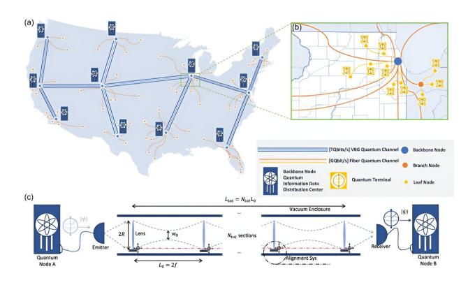
To make a quantum network a reality, researchers in Jiang Group at the University of Chicago Pritzker School of Molecular Engineering have proposed building long quantum channels using vacuum-sealed tubes with an array of spaced-out lenses. Credit: Jiang Group
