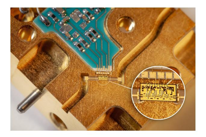
Close-up of the 89 GHz LNA MMIC integrated into the respective AWS microwave radiometer LNA module. Credit: Fraunhofer IAF
