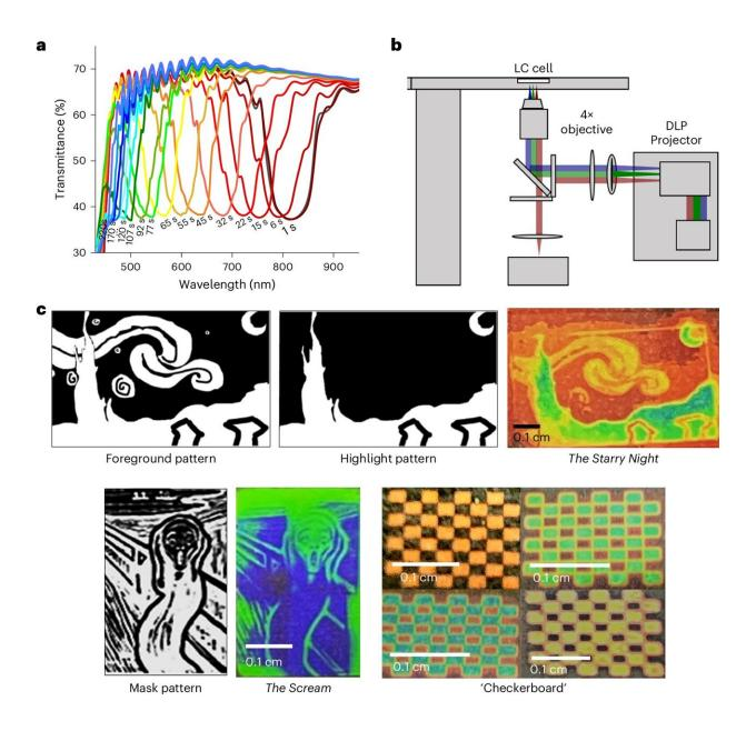
Transmittance spectra and DLP patterning of 5CB doped (S, S)-1 for multi-color image generation. Credit: *Nature Chemistry* (2024). DOI: 10.1038/s41557-024-01648-0
