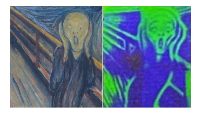
Researchers at Dartmouth and Southern Methodist University reproduced Edvard Munch's *The Scream* on a display screen made of liquid crystals (right) controlled by a chiral molecular switch they developed that reflects light in different colors. Credit: Ivan Aprahamian.
