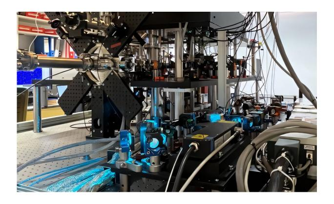
Part of the experimental set-up with the cylindrical oven and the apparatus for cooling of erbium atoms. The light from the cyan laser is used to trap the particles. Credit: IQOQI/Universität Innsbruck
