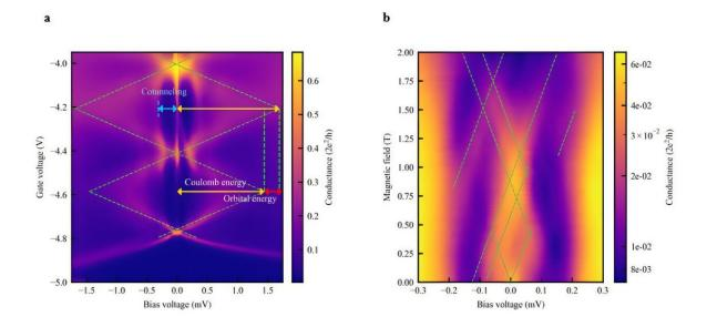
(a) Observed Coulomb diamonds, which are characteristic properties of quantum dots. Zero-bias peaks are observed at zero bias voltage in the figure. (b) Observed magnetic field dependence. The zero-bias peaks split in a complex manner, which is not observed in conventional Kondo effect. Credit: Adapted from *Nature Communications* (2024). DOI: 10.1038/s41467-024-53890-2
