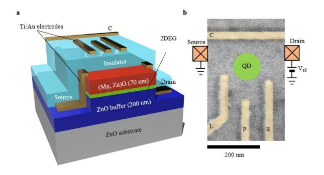
The structure of the zinc oxide (ZnO) device. A two-dimensional electron gas (2DEG) forms at the (Mg, Zn)O/ZnO interface. By applying voltages to the gate electrodes, we can confine electrons in a quantum dot. (b) An SEM image of the fabricated ZnO quantum dot device. The quantum dot is created in the circled region. Credit: Adapted from *Nature Communications* (2024). DOI: 10.1038/s41467-024-53890-2
