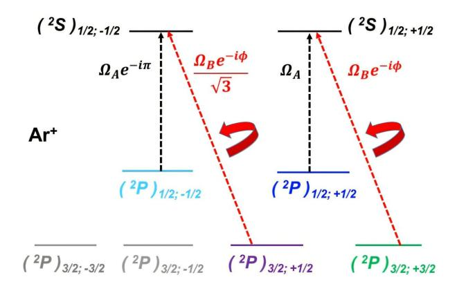
Schematic representation of the laser pulses to be applied to the Ar<sup>+</sup> parent ion subsystem within the entanglement detection protocol. Credit: *arXiv* (2023). DOI: 10.48550/arxiv.2312.05036
