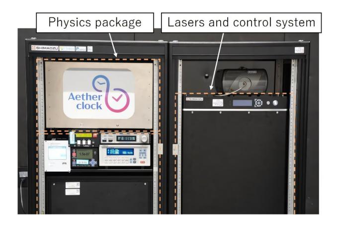
A compact optical lattice clock with a volume of 250 liters has been developed. The system includes a physics package for conducting spectroscopy on the clock transition within a vacuum chamber, lasers for manipulating atoms, a control system for clock operation, and an optical cavity that serves as a frequency reference for the lasers. Laser-cooled atoms are trapped in the optical lattice, and the clock transition frequency is measured with high precision in a low-
