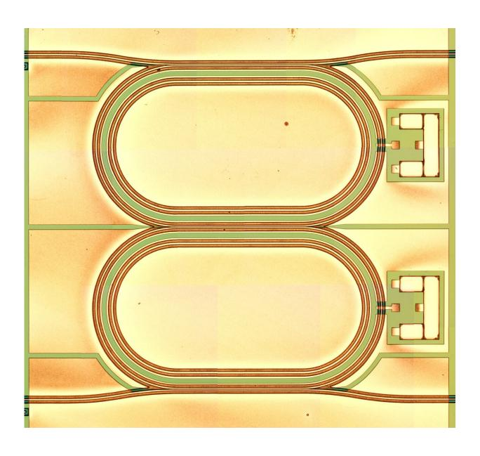
Image showing gold contacts where we bias each laser with DC current. Light is out-coupled from the racetracks using the directional-coupler waveguides along the straight section of either racetrack. Credit: *Physical Review Letters* (2025). DOI: 10.1103/PhysRevLett.134.023802
