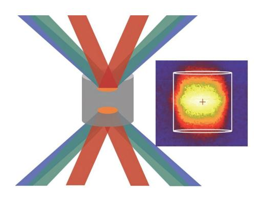
The NIF lasers overlap onto the millimeter-scale cylindrical silver foam target. The resultant heating creates X-rays, which are then imaged as shown on the right. Credit: Lawrence Livermore National Laboratory
