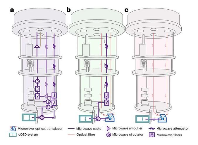
Comparison of conventional and optical qubit readout set-ups in a dilution refrigerator. Credit: *Nature Physics* (2025). DOI: 10.1038/s41567-024-02741-4
