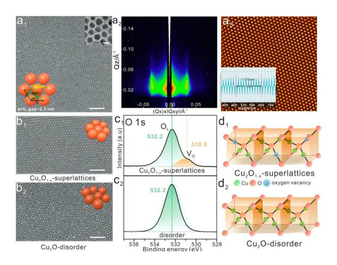
Characterization of oxygen vacancy properties generated by Cu<sub>2</sub>O<sub>1-x</sub> superlattice structures and corresponding disordered structures. Credit: Yao Chang
