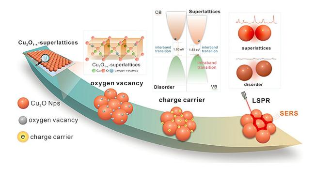
Changes in the properties of  $Cu_2O$  NPs after forming  $Cu_2O_{1-x}$  superlattice structures, and a schematic diagram of the mechanism for LSPR generation. Credit: Yao Chang
