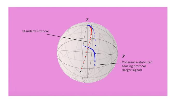
The qubit state decays toward the "north pole" of the sphere due to decoherence. Using the study's coherence-stabilized sensing protocol, the researchers temporarily counteracted the decay, leading to a larger sensing signal (y component) in the study's protocol (blue) than the standard protocol (red). Credit: Eli Levenson-Falk/USC
