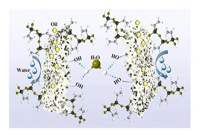
Mechanistic diagram of oil-water separation adsorption. Credit: *Scientific Reports* (2025). DOI: 10.1038/s41598-025-96059-7
