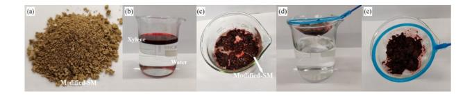
Oil pollution adsorption by modified sphagnum moss(modified-SM): (a) Macroscopic morphology of the modified sphagnum moss, (b) Oil-water mixture before adsorption, (c) Adsorption process showing adsorbed material, and (d, e) Separation of the material after adsorption. Credit: *Scientific Reports* (2025). DOI: 10.1038/s41598-025-96059-7
